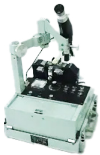
Fujikura FR-1 - 1977, the world's first fusion splicer
